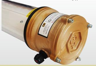
ZNP.X SERIES type fluorescent lamp comprises a lamp tube assembly ith two end caps. The housing consists of a transparent polycarbonateube with polycarbonate end caps. The electronics are located in the main body. Both end caps connected together by two 'mm diametertie bars, therefore compressing the tube and caps. The equipment is intended for fixed installation. The equipment has normal fluorescent lamp, led fluorescent lamp and emergency kit variations.
